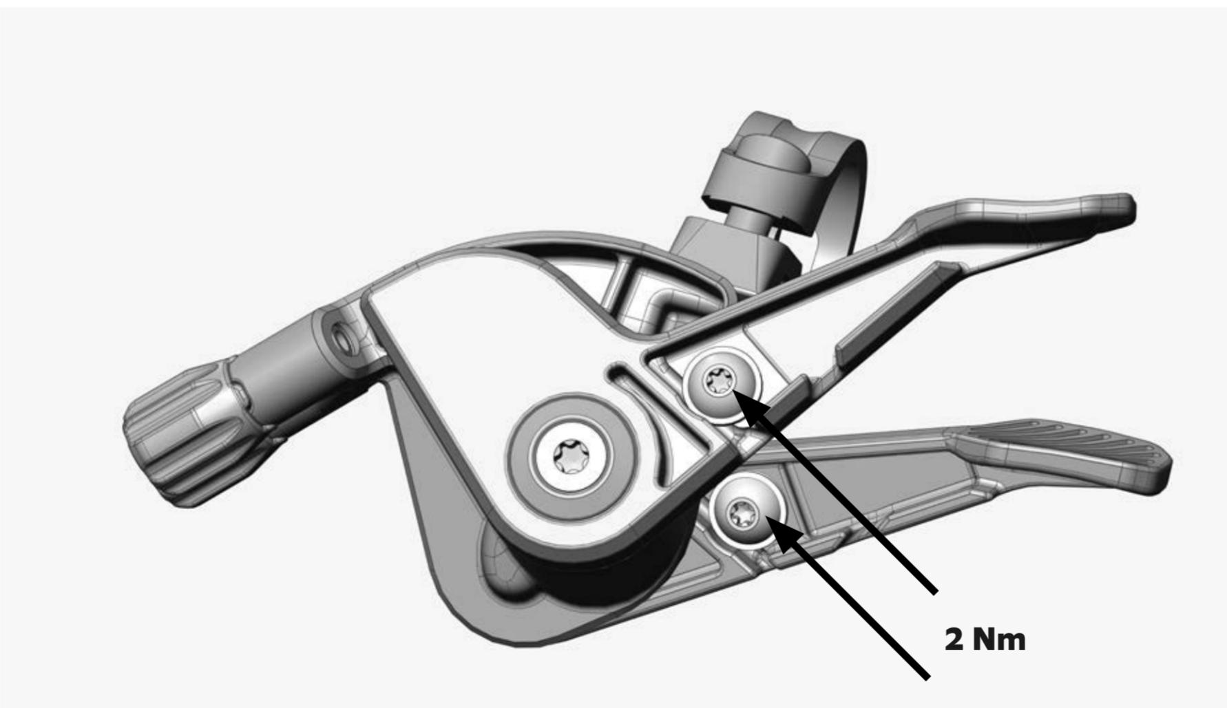
Check if the barrel adjusters are in their middle position by rotating them. Lead the innercable through the correct shifter and fix them with the screws. Tighten them with 2 Nm.
