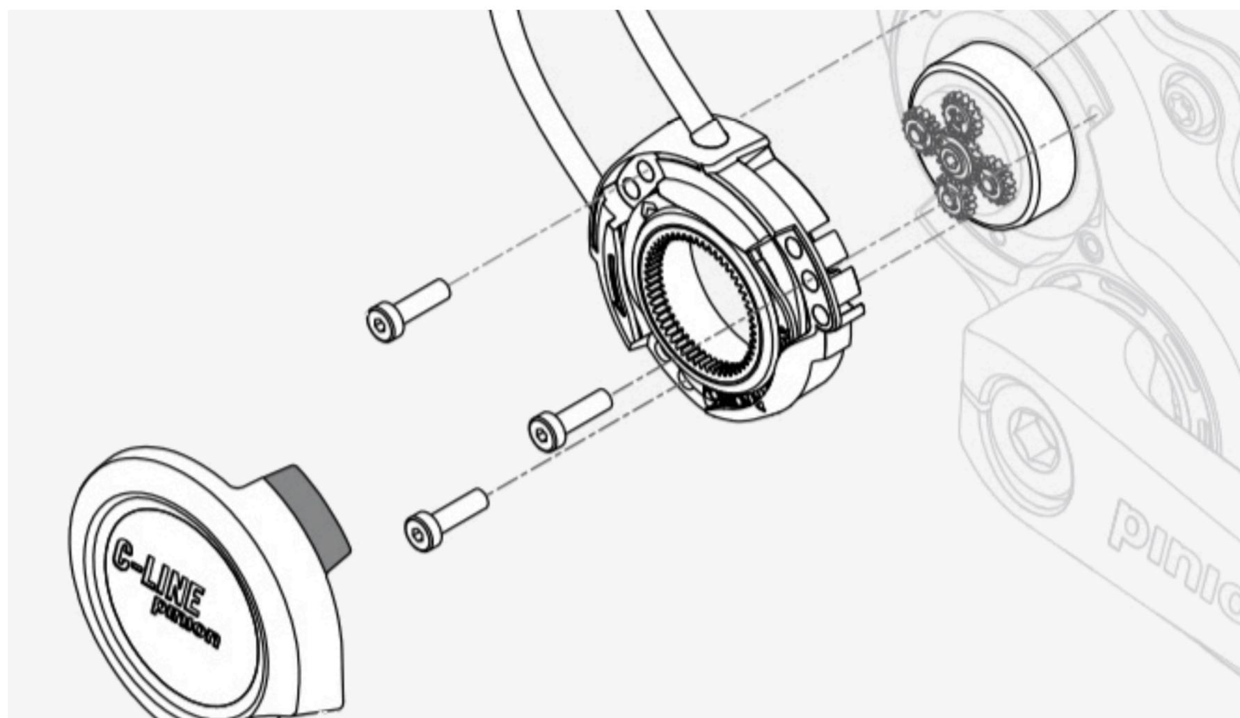
Remove the C-line plastic cap, loosen the 3 screws and remove the shift box. Leave the bowden cables in place, only remove the inner cables. You will need the three screws.
