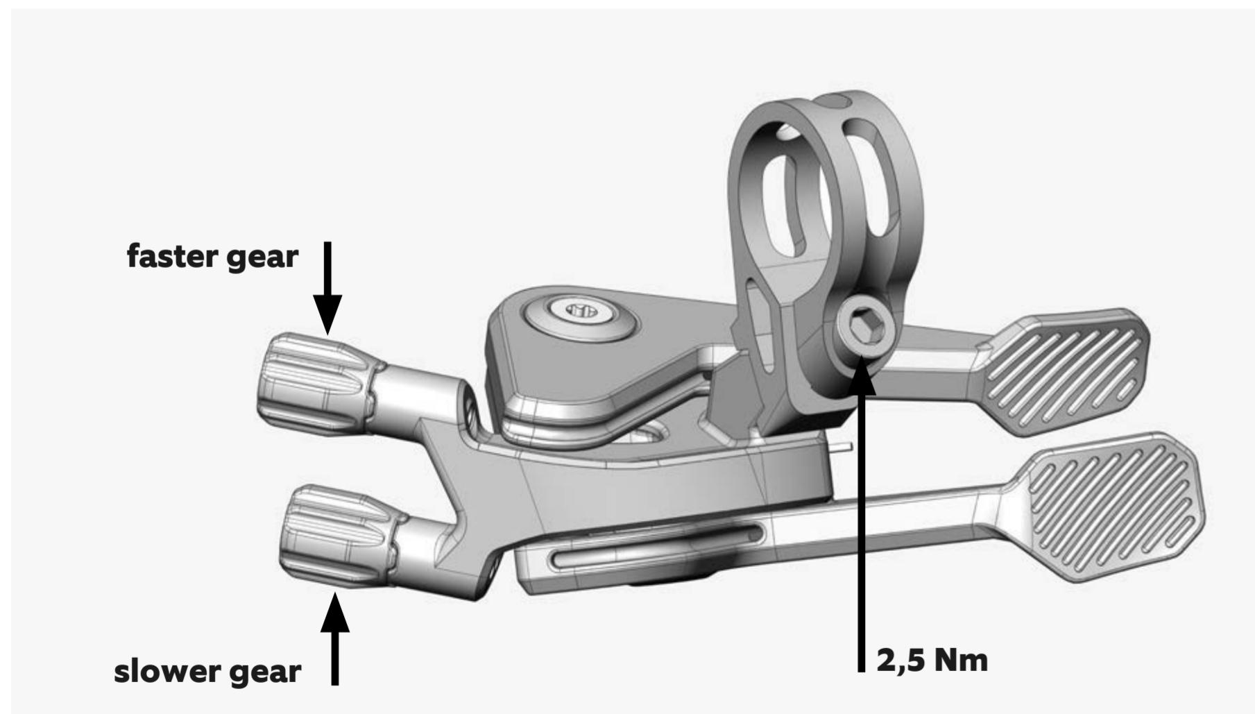
Fix the trigger shifter to the handlebar. Tighten the screw with 2,5 Nm. Lead the correct innercables through the barrel adjusters.
