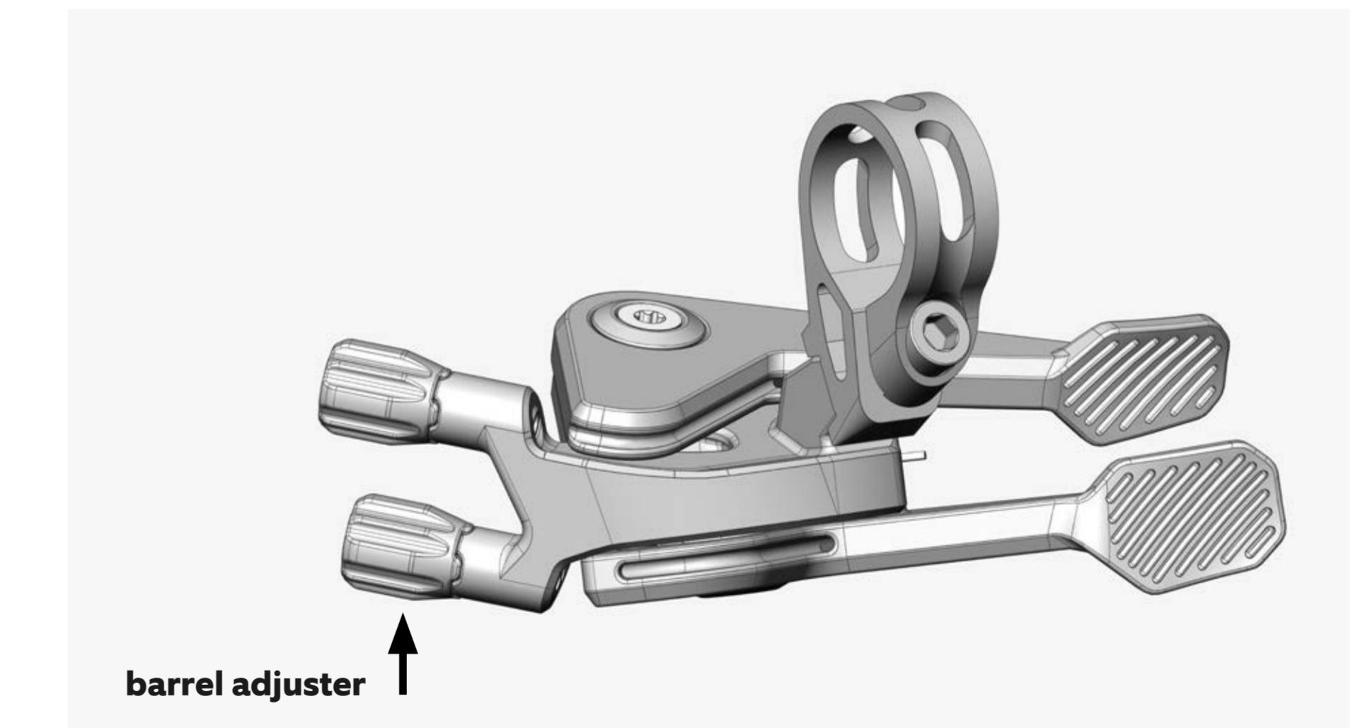
Rotate the barrel adjusters both a bit outward to add some tension. If there is a grinding sound while shifting, rotate the opposite adjuster inwards and the other outwards, till there is no sound and shifting is smooth.
