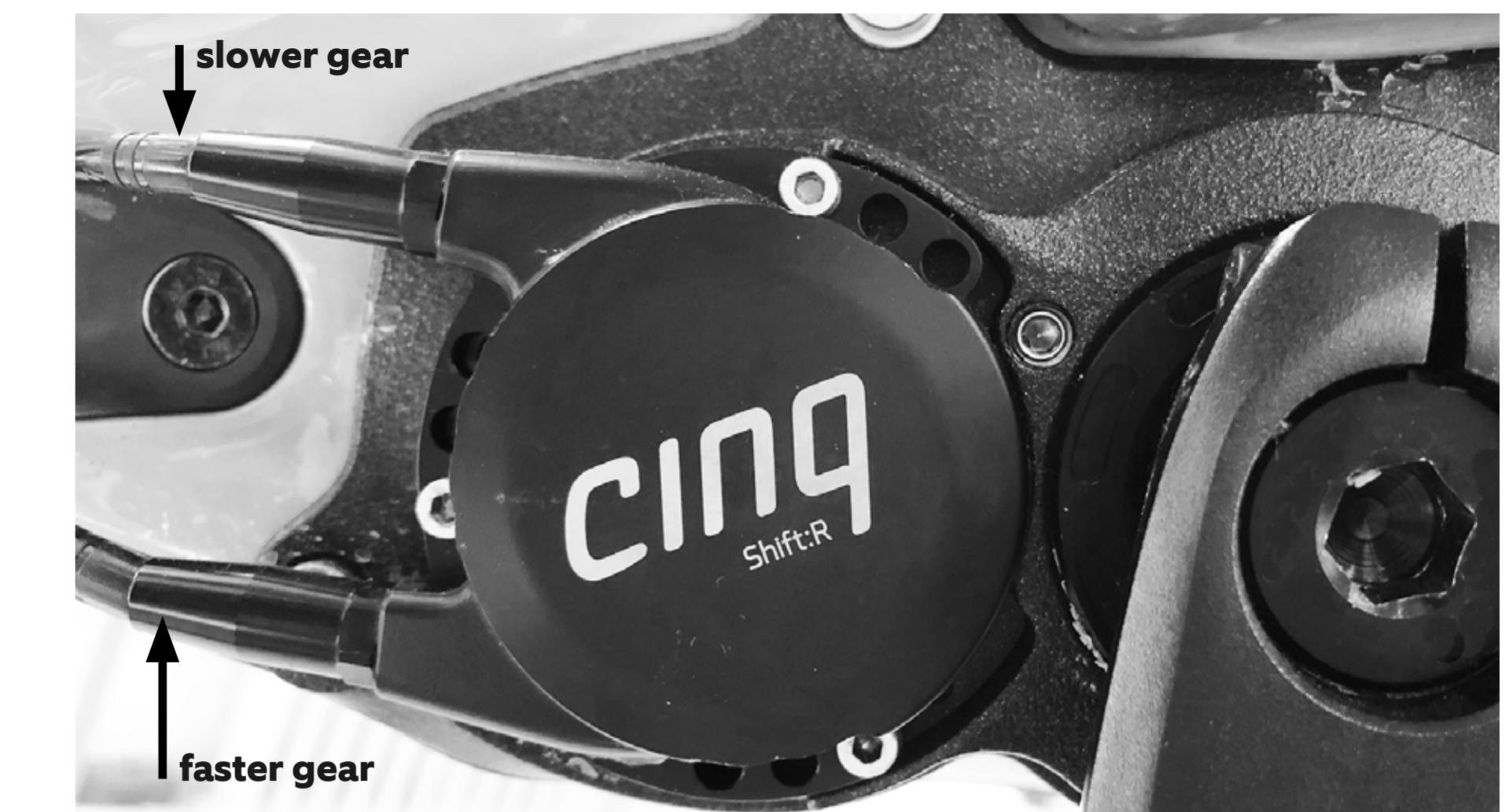
Lead the inner cables of the Cinq into the bowden cables and Install the Cinq shiftbox on the Pinion gearbox with the same screws. Tighten with 1.5Nm.
