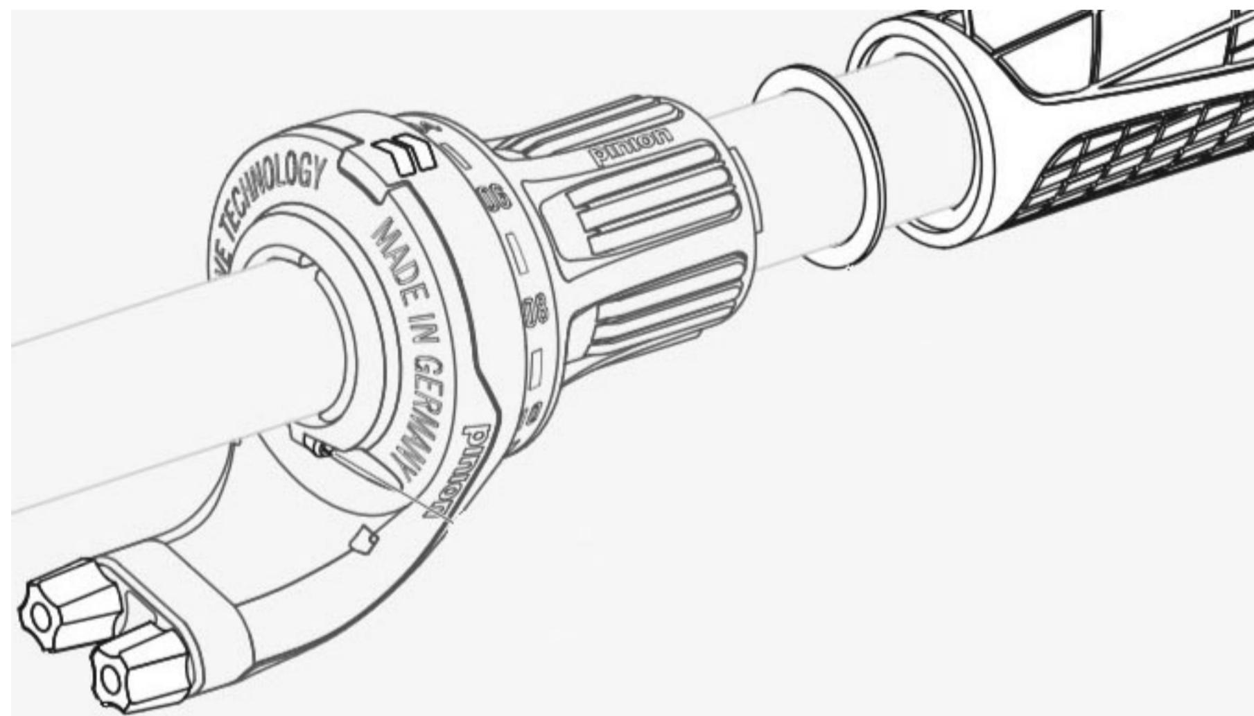
If you have a Pinion DS2 rotary shifter installed you will need to remove the grip and shifter. Loosen the shift cables.
